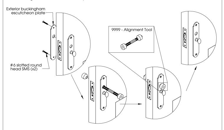
5) Install spindle into exterior knob until it bottoms out as shown below. Secure using the set screw in the knob.
